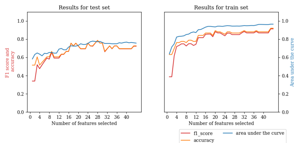
Figure 6. Results for the test (left) and training set (right) of the Linear Discriminant Analysis Classifier, showing the performance metrics, f1-score, accuracy, and area under the curve, plotted against the number of features used for the model.
